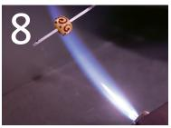
Create a reduction flame by reducing the oxygen, increasing the propane, or both. Gently reheat the bead at the tip of the flame.
