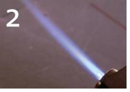
Adjust to a small oxydizing flame.
