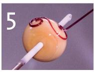
The stringer should be at the right edge of the flame and never inside the flame.
