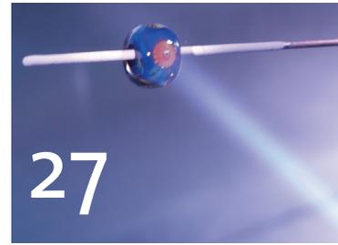
27 Cool until the glow is gone, and then reintroduce the bead at the tip of flame to strike.
