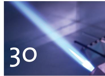
30 Cool the bead until the glow is gone. At the same time create a medium reduction flame by reducing the oxygen, increasing the propane, or both.
