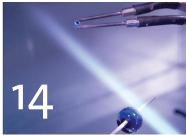
14 Spot heat the base bead where you want to apply the murrini while preheating the murrini chip at the tip of the flame.
