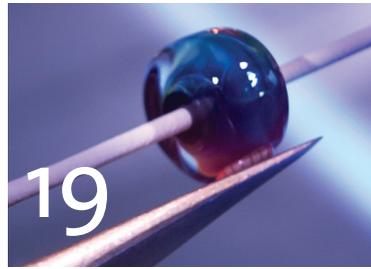
19 Repeat until murrini is almost flushed with the surface of the base bead.
