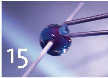
15 Position and apply murrini chip on base bead, press in very slightly with the tips of the tungsten-tip tweezers.
