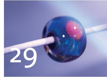
29 Gently reheat and cool slightly multiple times to bring out desired colors. Bathe the entire bead evenly in the flame for insurance heat until it barely glows.
