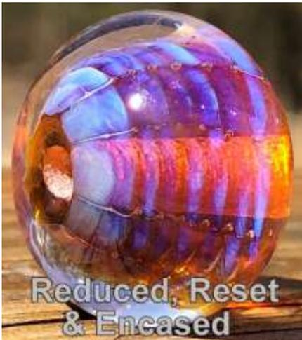
Reduction colors contain silver dissolved in the glass matrix as Silver Oxide ( $\text{Ag}_2\text{O}$ ). Upon exposure to a flame deficient in oxygen, the  $\text{Ag}_2\text{O}$  gives up its oxygen to the flame, leaving behind a thin layer of metallic silver. This metallic layer can be left on the surface or encased in clear glass.
